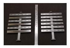
Phase I antennas (an 18-slot array, a 12-slot array, and a 36-slot array) that were successfully designed, simulated, built, and tested.
