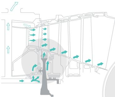
Flownex<sup>®</sup> includes a comprehensive rotating component flow library for analyzing the coolant rotational flow field inside the gas turbine engine, also referred to as the secondary air system. The Flownex<sup>®</sup> flow network approach leads to much faster and more cost- effective baseline designs for these systems since the number of expensive, detailed simulations are minimized.
