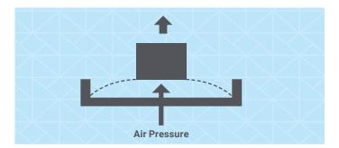
Origin's pneumatic separation mechanism applies much less separation force: the membrane gradually peels off each cured layer as the build platform goes up.
